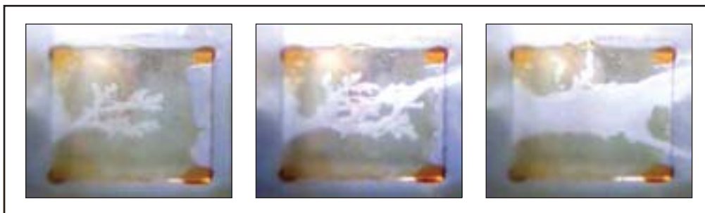
Figure 17. This series show the rapid progression of channeling flow cleaning mechanism
