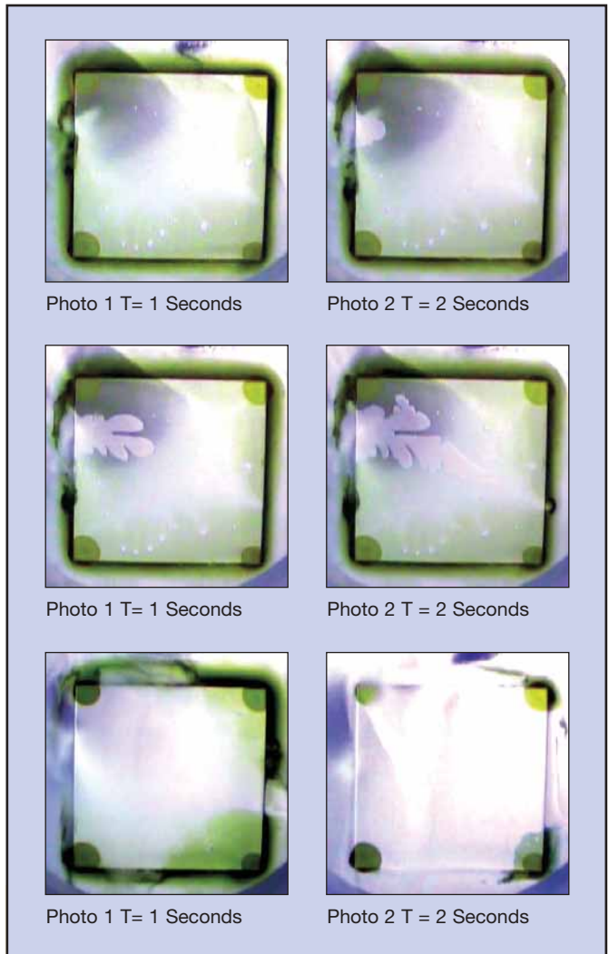
Figure 7. Sequence of the Channeling Cleaning Process.
