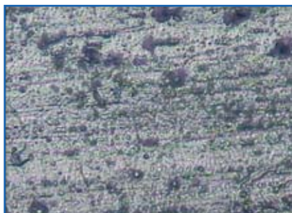
Figure 8. Slightly anodized AL. Needs no pre-aging.
