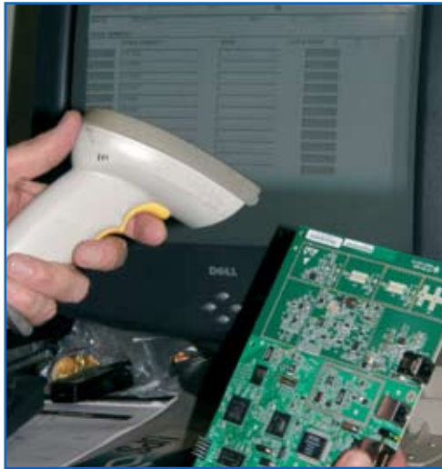
Figure 1. Work-in-process is tracked via bar codes throughout the production process.
