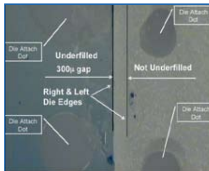
Figure 12. 300 \mu m gap. Die adhesive was used to maintain the gap between the substrate and the glass die.
