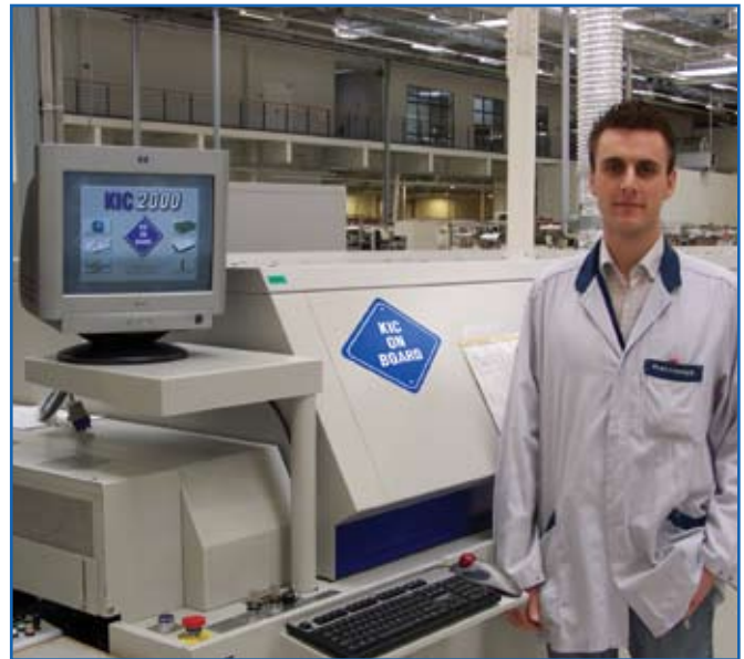
Figure 1. The experiments were conducted using a Heller 1912 EXL reflow oven and a SlimKIC 2000 profiler with Auto-Focus optimization software.
