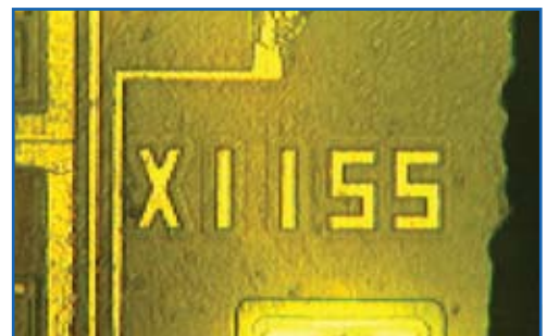
Figure 2. A metallurgical microscope set up to capture images of the die inside the package captures this close-up of a die's identifying marks.
