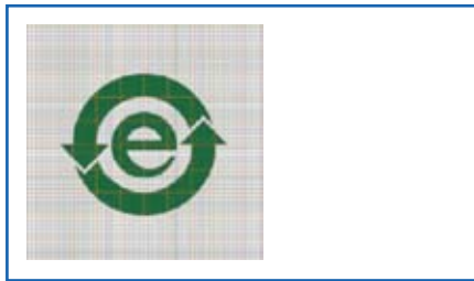
Figure 2. Symbol for marking of (Green) EIP which don't contain any banned hazardous substances 14 .
