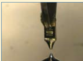
Figures 1: Testing chip components for solderability. Images taken from a video provided courtesy Gen3 Systems.
