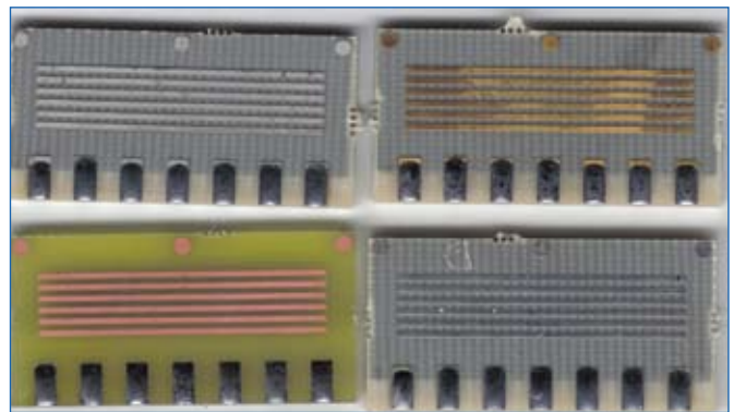
Figure 2: Printed board samples after testing with the wetting balance: top left Sn (tin), top right Au (gold/nickel), bottom left Cu (copper OSP), bottom right Ag (silver).
