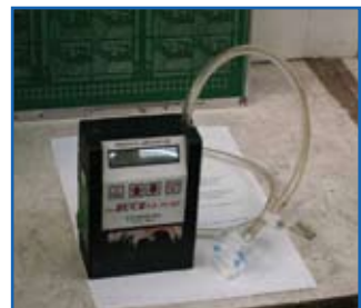
Figure 1. Close-up of the air monitoring/sampling device used by production staff.
