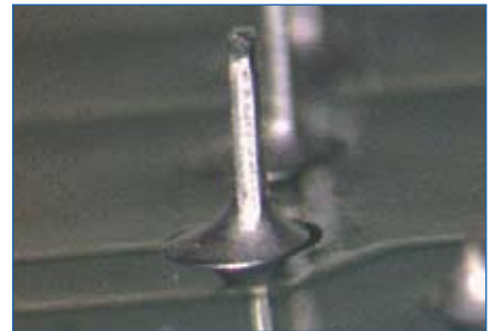
Figure 4. A leaded device with tin/lead plated leads wave soldered with tin/copper/nickel alloy onto an immersion gold/electroless nickel printed board.
